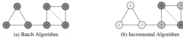
Fig. 1. Calculated node centralities with edge \{(4, 6)\} added. Dark grey nodes affected by addition of edges. Light grey nodes centralities need to be calculated due to their neighbourhood with affected nodes.
